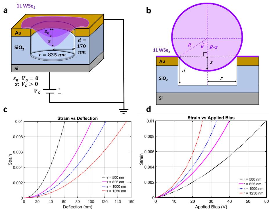
**Figure 2** Strain calculations from electrostatic-induced deflection of suspended monolayer WSe<sub>2</sub>. Schematic diagrams of a suspended WSe<sub>2</sub> monolayer over patterned-hole substrate and straining approach (a) and a circumferential strain model of suspended WSe<sub>2</sub> monolayer (b). Calculated strain as a function of monolayer deflection (c) and strain as a function of applied bias (d) assuming a semi-spherical monolayer deflection geometry.
