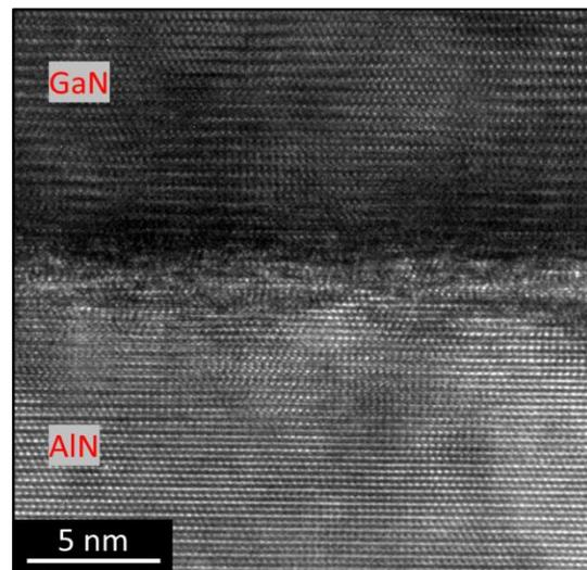
Figure 1 HRTEM of the wafer bonded GaN-AlN interface. ~1.5 nm interface can be observed due to reconfiguration of atoms after high temperature annealing.
