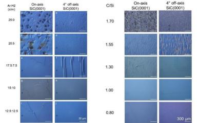
Nomarski micrographs for RE SiC films on epitaxial graphene (EG) substrates using various Ar:H<sub>2</sub> carrier gas ratios and a fixed C/Si ratio of 1.55 (left) and various C/Si ratios with a fixed Ar:H<sub>2</sub> ratio of 17.5:7.5 slm (right). Highest quality films are found with C/Si < 1.55 and Ar:H<sub>2</sub> < 20:5.
