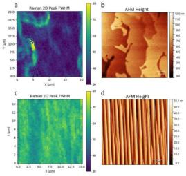
Raman EG 2D peak FWHM maps (a, c) and AFM height images (b, d) of representative samples of ~1 ML EG grown on nominally on-axis, semi-insulating 6H-SiC(0001) (a, b) and ~4-5 ML EG on  $4^{\circ}$ -offcut, N-type 4H-SiC(0001) (c, d). FWHM color scale is measured in cm<sup>-1</sup>.
