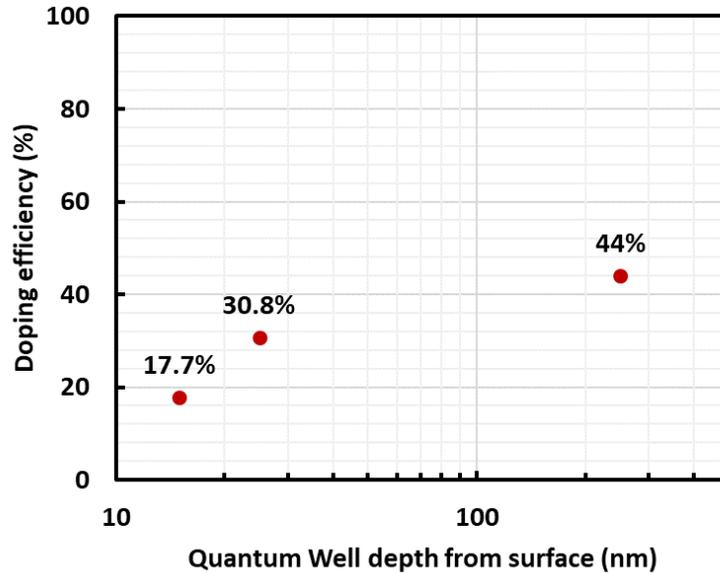
Fig. 2. Plot of doping efficiency of n-type Silicon dopants vs. depth of a 25nm wide InAsSb QW on GaSb substrate. As the QW is brought closer to the surface, the doping efficiency reduces, indicating the presence of a surface depletion layer (negative charges). This would indicate the fermi-level at the surface is pinned within the gap of the semiconductor.
