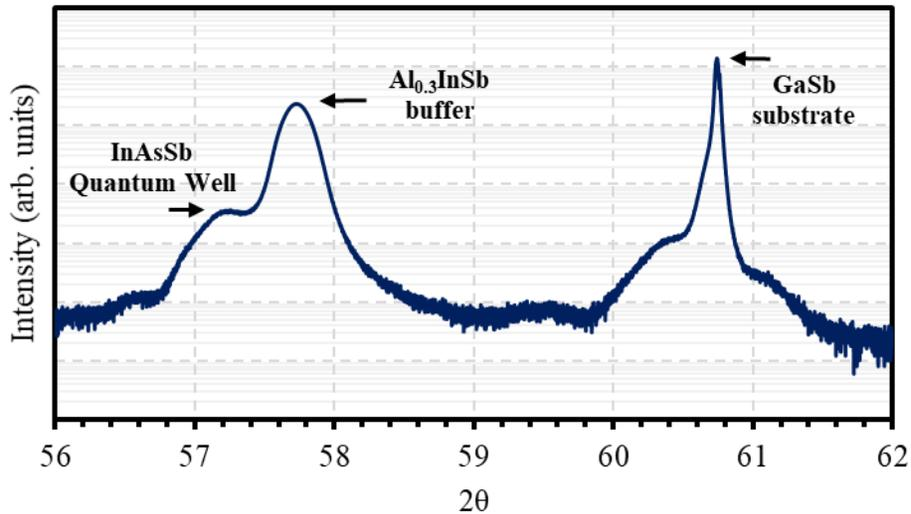
Fig. 3. X-Ray diffractogram of an InAsSb QW grown on an Al<sub>0.3</sub>InSb barrier layer on a GaSb substrate. The diffraction peak for the QW corresponds to a composition of InAs<sub>0.2</sub>Sb<sub>0.8</sub>. This diffractogram in conjunction with *in-situ* Reflection High Energy Electron Diffraction (RHEED) indicates that the quantum well is strained compressively on the Al<sub>0.3</sub>InSb buffer/barrier layer.
