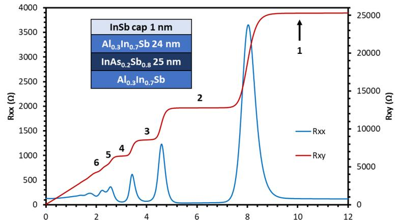
Fig. 1. Magneto-transport measurements of InAsSb QW at 2K
