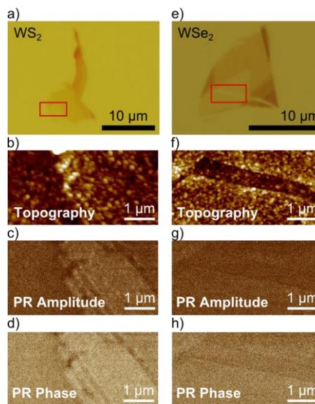
**Figure 1.** Optical images (a, e), and simultaneously captured topography (b, f), PR amplitude (c, g) and PR phase (d, h) images taken on WS<sub>2</sub> (a, b, c, d) and WSe<sub>2</sub> (e, f, g, h). The red box in a and e indicate the location of the PFM images taken below.
