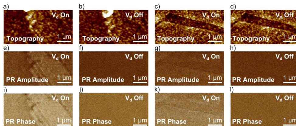
**Figure S2.** PFM images of WS<sub>2</sub> (a, b, e, f, i, j) and WSe<sub>2</sub> (c, d, g, h, k, l) taken with the drive voltage ( $V_d$ ) applied (a, c, e, g, i, k) and not applied (b, d, f, h, j, l). The topography (a - d), PR amplitude (e - h) and PR phase (i - l) images in each case are taken simultaneously. The disappearance of the contrast when  $V_d$  is not applied indicates that there are no scanning artifacts.
