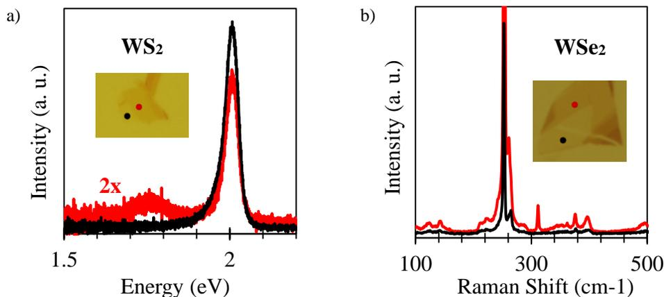
**Figure S1.** a) Photoluminescence (PL) measurements of WS<sub>2</sub> monolayer (black) and multilayer (red) regions scanned in Figure 1. The strong, single peak in the PL signal indicates that it is monolayer [S1]. b) Raman shift of WSe<sub>2</sub> monolayer (black) and multilayer (red) region scanned in Figure 1. The absence of the peak around 310 cm<sup>-1</sup> in the black curve indicates that it is monolayer [S2].
