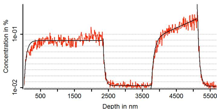
**Figure 2.** Si-doping profile in an InP nanowire as obtained by Atom Probe Tomography. Muraki-type fits were used to describe the quality of the doping interfaces.
