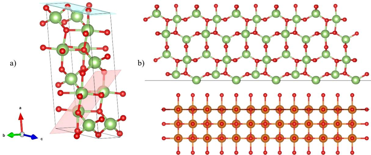
**Fig. 1** a) Monoclinic unit cell of  $\beta\text{-Ga}_2\text{O}_3$  with the (100) and (-201) planes highlighted in blue and red, respectively. b) The planar mismatch between  $\beta\text{-Ga}_2\text{O}_3$  and MgO. The (100) plane of both crystals is indicated by a black line.
