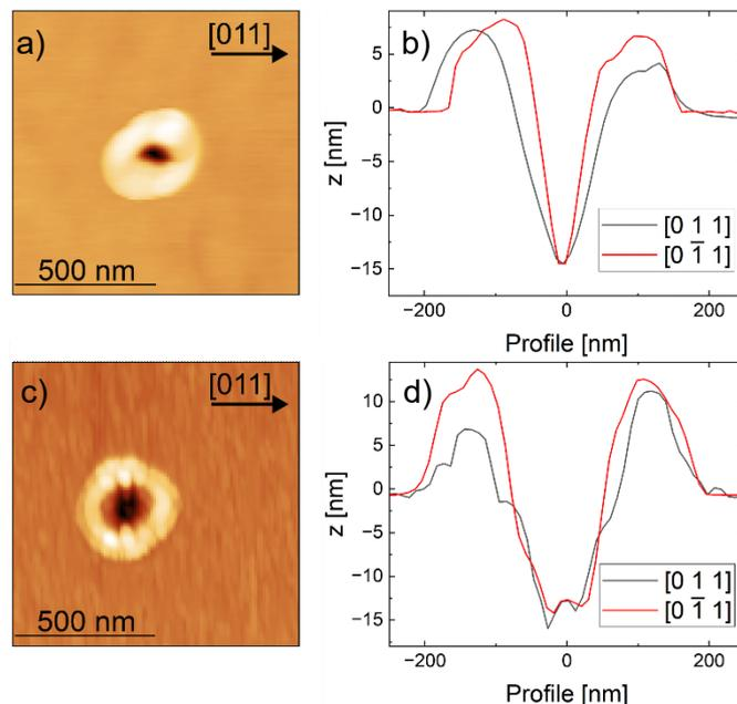
**Fig. 3:** AFM images and profiles for nanoholes etched with approximately 2 ML of Al ( a) and b)) and 2 ML of In ( c) and d)). The etching temperature  $T_{\text{etch}}$  was in both cases 435°C. Holes etched with Al are significantly more elongated along the [011] direction as can be seen from the image a) and the line scans along the high symmetry directions b).
