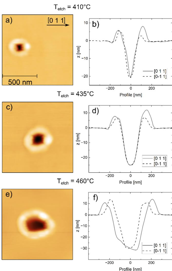
**Fig. 2:** AFM images and line profiles for samples overgrown with 50 nm  $\text{In}_{0.52}\text{Al}_{0.48}\text{As}$  and etched at 410°C ( a) and b)), at 435°C ( c) and d)), and at 460°C ( e) and f)), respectively. Etching was performed with 4.1 ML of  $\text{InAl}$ . The size of the AFM images is  $1 \times 1 \mu\text{m}^2$ .
