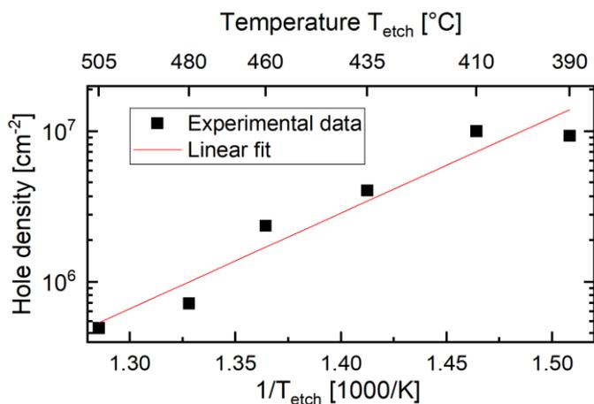
**Fig. 1:** Surface density of etched nanoholes vs. the inverse etching temperature  $T_{\text{etch}}$ . Data points were generated by counting nanoholes at 2,000x magnification in an SEM evaluating at least 40 nanoholes per temperature.
