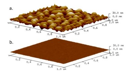
AFM scans of two aluminum layers grown on  $In_{0.75}Ga_{0.25}As/In_{0.53}Ga_{0.47}As$  (6nm/100nm) on the InP(001) substrate. In both cases, the nominal thickness of the Al layer was 10 nm.
