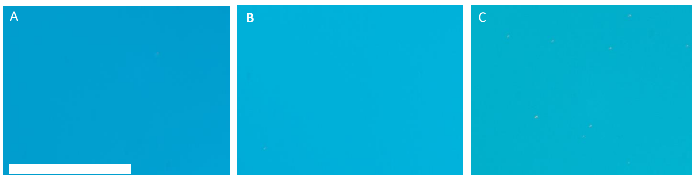
Figure 4 Normaski microscope Images of sample surfaces A, B & C for X=0.0, 0.05 & 0.15 Al_xGa_{(1-x)}As_{(1-y)}Bi_y alloys respectively with 300\mu m scale bar.
