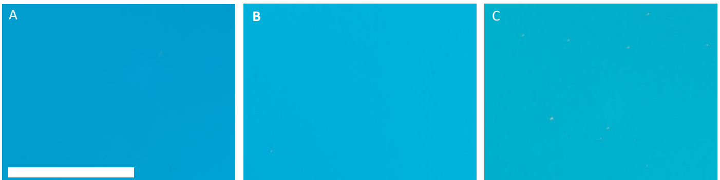
Figure 4 Normaski microscope Images of sample surfaces A, B & C for X=0.0, 0.05 & 0.15 Al_xGa_{(1-x)}As_{(1-y)}Bi_y alloys respectively with 300\mu m scale bar.
