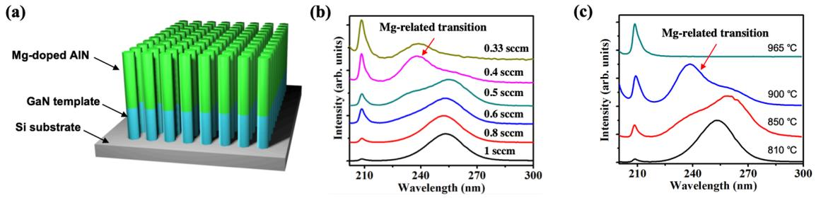
Figure 1. (a) schematic of Mg-doped AlN nanocrystals grown on Si substrate. Room temperature photoluminescence of Mg-doped AlN nanocrystals grown under (b) varying nitrogen flow rate and (c) varying substrate temperature. The pronounced Mg-acceptor related transition can be clearly measured (indicated by the red arrow).
