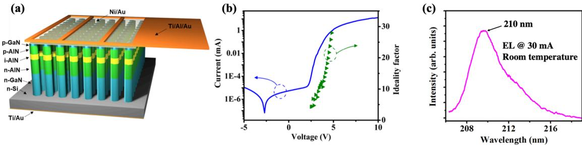
Figure 2. (a) schematic illustration of the fabricated large area AlN deep UV LED. (b) Current-voltage (I-V) characteristics measured at room temperature. (c) Room-temperature electroluminescence (EL) spectrum measured from AlN LEDs.
