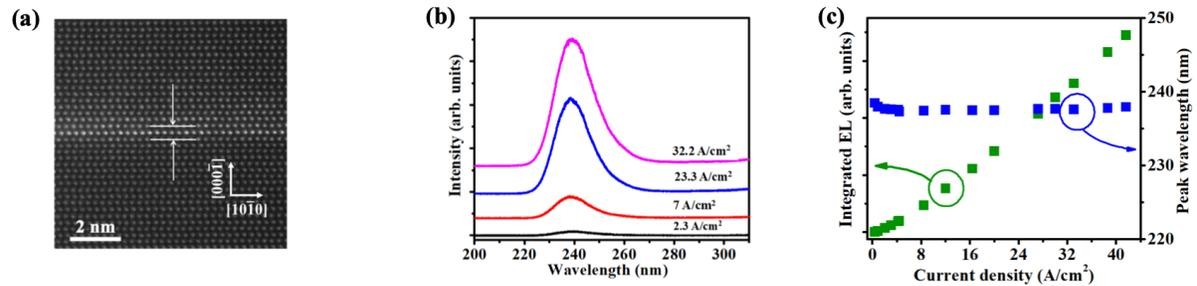
Figure 3. (a) STEM-HAADF images of one monolayer GaN quantum disk embedded in AlN matrix. (b) Electroluminescence spectra measured under injection currents from 2.3 A/cm<sup>2</sup> to 32.2 A/cm<sup>2</sup> for the monolayer GaN LED. (c) Variations of the integrated electroluminescence intensity (green) and peak position (blue) vs. injection current. The measured device size is 300  $\mu\text{m}$   $\times$  300  $\mu\text{m}$ .
