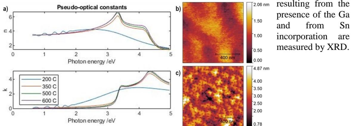
Figure 1. Effect of growth temperature on homoepitaxial Si film quality, demonstrated by a) changes in the pseudo-optical constants of 500nm Si films on float-zone Si wafers, and the AFM-determined surface features of homoepitaxial Si films grown at b) 600°C and c) 350°C.
