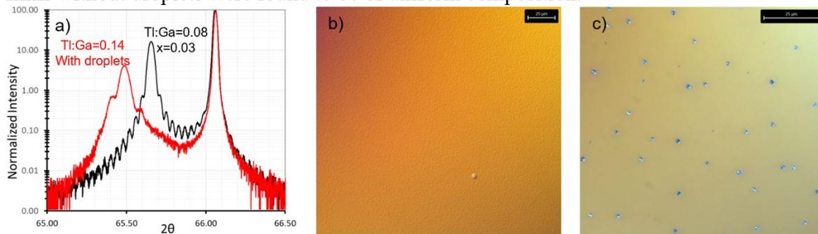
Figure 1: a) HRXRD 004  $2\theta$ - $\omega$  scans of a  $\text{Tl}_{0.03}\text{Ga}_{0.97}\text{As}$  film grown with low Tl:Ga BEP ratio (black) and a TlGaAs film grown with high Tl:Ga (red). The high Tl:Ga BEP ratio produced films with compositional variation and surface droplets. b) and c) show DIC optical images of the surface of each sample respectively. Samples were grown at  $190^\circ\text{C}$ .
