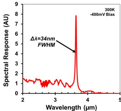
Figure 1. RCE-PD with a 34nm FWHM spectral linewidth at 3.6μm resonance.
