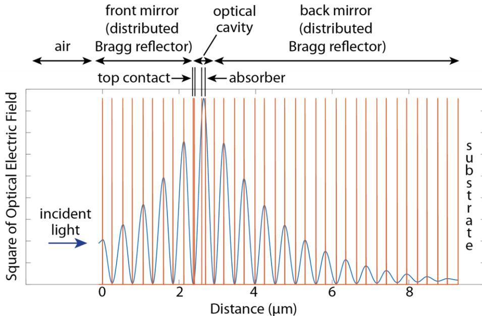
Figure 4. Epitaxial Design of the all-epitaxial RCE-PD is non-trivial. The optical absorber must be placed on an anti-node of the optical electric field within the resonant cavity to ensure the highest level of MWIR detection. Furthermore, the narrow-bandgap top contact layer must be placed on a node of the optical electric field to ensure minimal photon absorption within the top contact.
