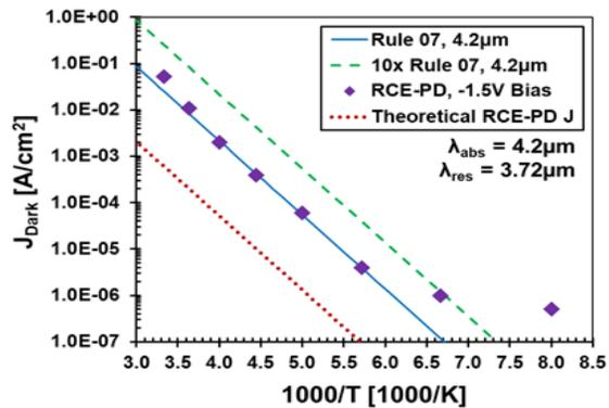
Figure 2. Dark current of a 3.72μm RCE-PD matches Rule07 at absorber resonance.
