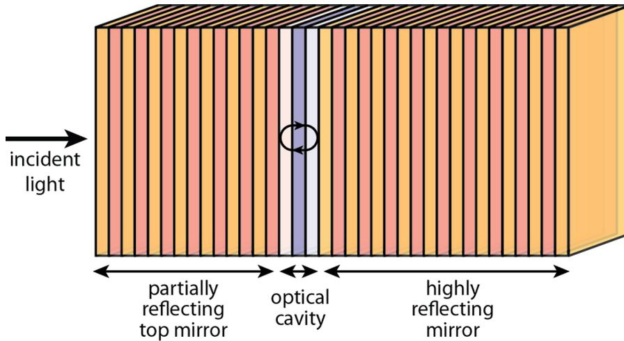
Figure 3. Schematic of an all-epitaxial RCE-PD. The highly reflecting back mirror and the partially reflecting top mirror are deposited via MBE as a distributed Bragg reflector consisting of  $\lambda/4$  layers of two differing, large bandgap III-V materials lattice-matched to the substrate (GaSb in this case). Between the reflectors, an optical cavity is deposited consisting of two large bandgap spacer layers (also lattice matched) and a thin MWIR optical absorber.
