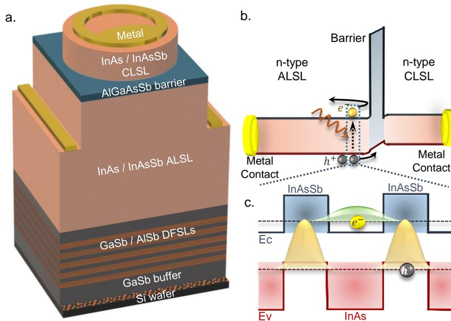
Figure 3: (a) Schematic of the InAs/InAsSb type-II SL nBn structure grown on top of the GaSb/AlSb/Si buffer, using AlSb/GaSb dislocation filters. (b) Diagram of the full device's bandgap structure showing the barrier layer which blocks the flow of electrons. (c) InAs/InAsSb SL bandstructure with first electron and hole energy levels and wavefunctions. The dashed lines represent the minibands formation.
