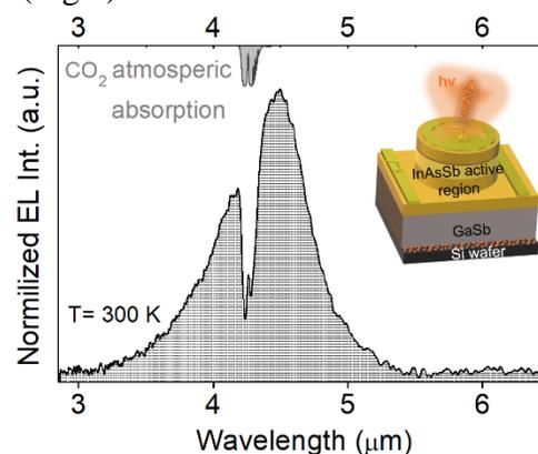
Figure 2 Room Temperature EL measured from the LED peaking at 4.46  $\mu\text{m}$ .
