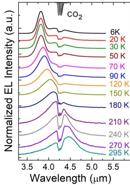
Figure 5: The temperature dependent normalized EL emission spectra obtained from the InAsSb p-i-n LED grown on top of the GaSb/Si buffer layer using 190 mA, 1kHz and 50% duty cycle.
