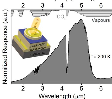
Figure 1 Photoresponse measured from the nBn detector grown on Si at 200 K.
