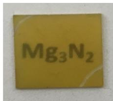
Figure 1. Photograph of capped  $\text{Mg}_3\text{N}_2$  film 800 nm thick with chemical formula visible on paper below.
