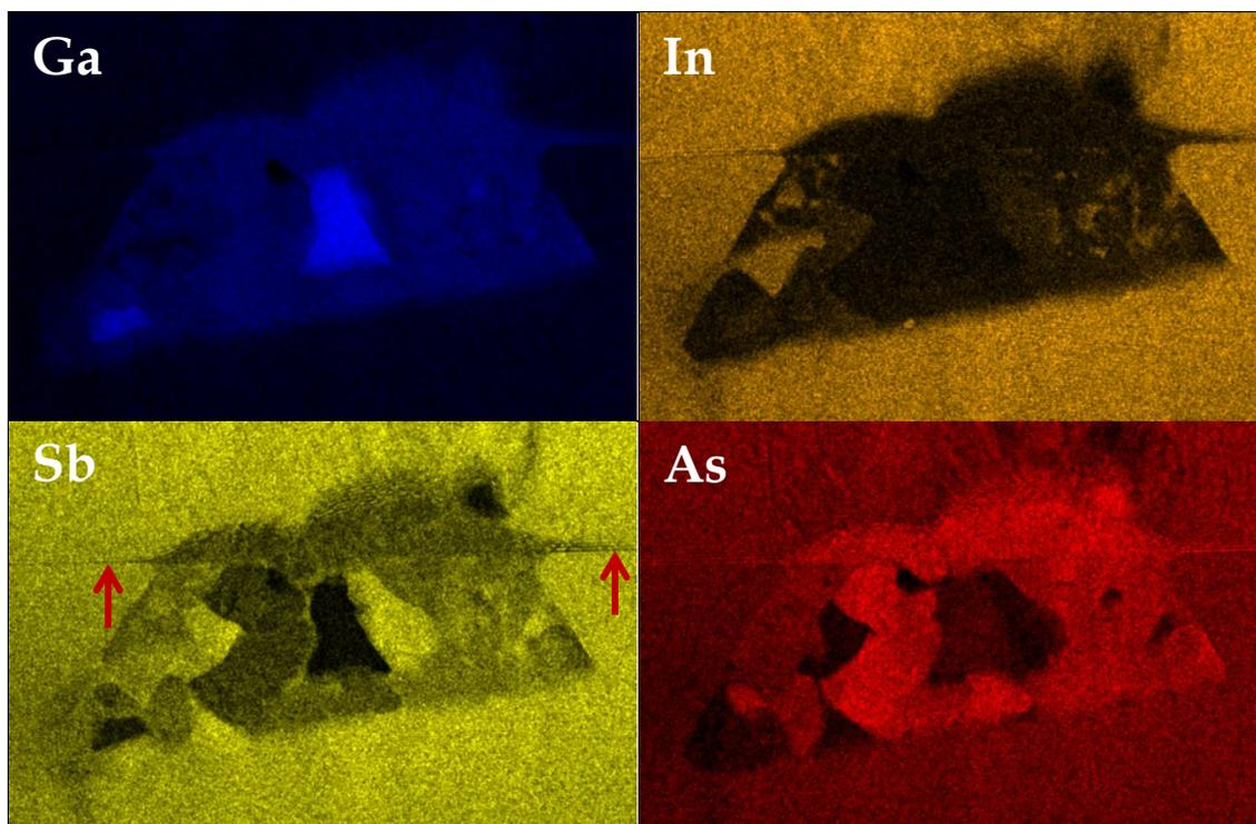
Figure 3. TEM EDS mapping images of the sample shown in figure 1. Note that in the center of the defect there is practically pure Ga and around it we can see mainly GaAs and some InSb although our structure is InAs/GaSb. The two red arrows indicate the growth front at the moment of the Ga droplet landings. The highlighted layer there is Ga rich due to gallium migration from the droplet.
