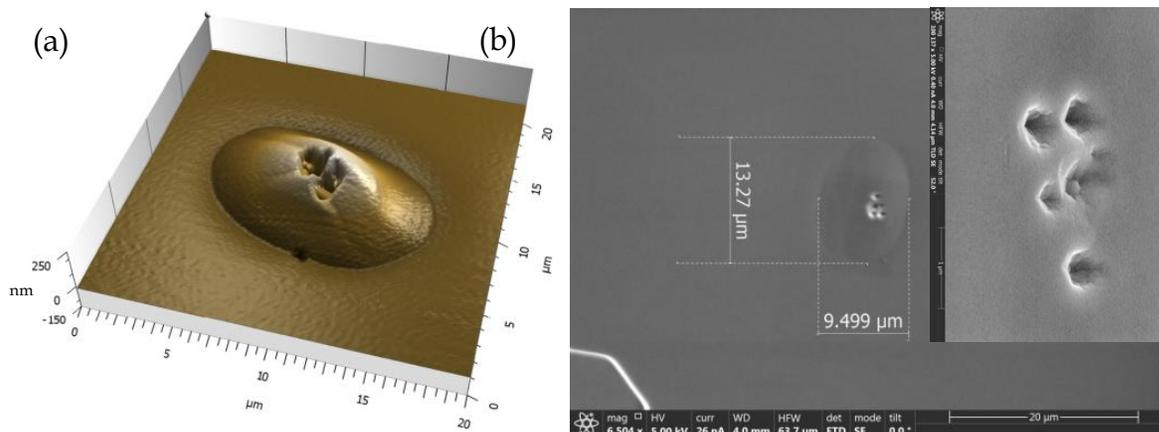
Figure 2. (a) AFM measurement of a typical defect. The length of the defect in the  $[0-1-1]$  direction is in the order of 10-15  $\mu\text{m}$  while the length in the perpendicular direction  $[01-1]$  is always shorter (probably due to lower ad-atom mobility at this direction in this material) (b) SEM images of the defect shown in figure 1. The pits in the center of the defect are seen also in the TEM cross section.
