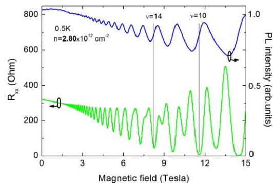
Fig. 2: Simultaneously recorded B-field induced PL intensity oscillations (top) along with magneto-transport oscillations (bottom) from an AlGa<sub>N</sub>/Ga<sub>N</sub> 2DEG.
