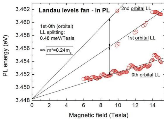
Fig. 5: Landau level fan obtained from evaluation of magneto-PL data (c.f. Fig. 1). From the separation of the LLs an effective electron mass of  $0.24 m_0$  is extracted.
