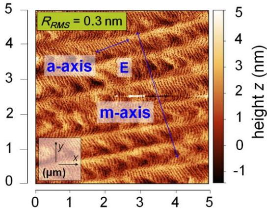
Fig. 3: Surface morphology scanned by AFM of a  $5 \times 5 \mu\text{m}^2$  section of the AlGaIn/GaN heterostructure showing no surface defect originating from dislocations. The ripple structure originates from monolayer steps (260pm) resulting from the crystal miscut with respect to the a- and m-directions (from [2]).
