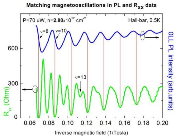
Fig. 7: Magneto-PL and -transport data plotted vs. the inverse magnetic field. Despite the shift between the respective minima and maxima, the oscillation frequency is proportional to the 2D density, yielding identical values for the spectroscopic and electrical measurements.
