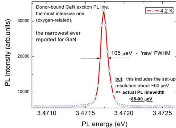
Fig. 4: Donor-bound exciton PL originating from the MBE-grown 1 μm thick GaN buffer with a linewidth of  $< 100 \mu\text{eV}$  proves the excellent crystalline quality of the epitaxially-grown layer stack.
