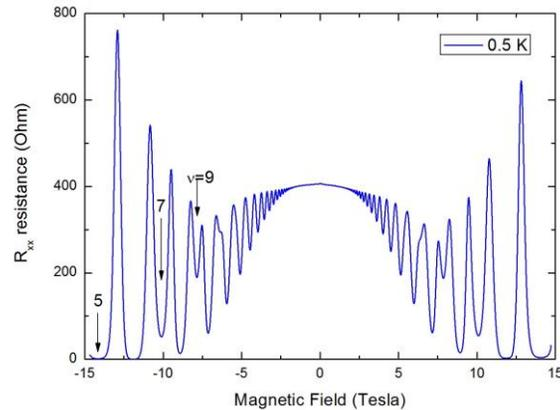
Fig. 6: Longitudinal magneto-resistance of the AlGaIn/GaN 2DEG without illumination. At high magnetic fields pronounced zero-resistance states and odd filling factors are identified.
