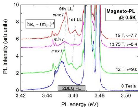
Fig. 1: The PL spectral band from the 2DEG at the AlGa<sub>N</sub>/Ga<sub>N</sub> heterojunction detected at  $\sim 3.45$ eV. Characteristic splitting of the band into Landau levels in a magnetic field is visible, along with prominent changes in the intensity.
