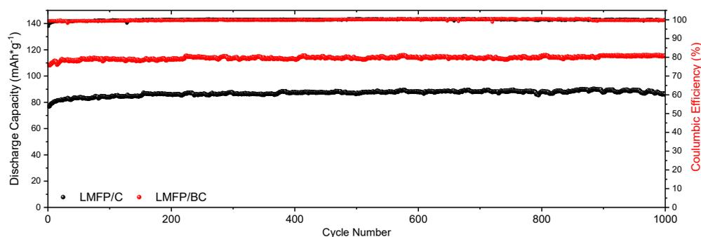
Figure. 2 Cycling performances of both LMFP samples at 1 C-rate at 25 °C between 2.4 and 4.5 V.
