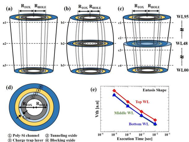
**Fig. 1.** Schematics of vertical GAA structure varying etching and oxidation process with (a) trapezoid, (b) entasis and (c) iterated trapezoid structures. (d) Top view for GAA in 3D CTF (e) Experimental data showing variations of erase speed along the WLs.
