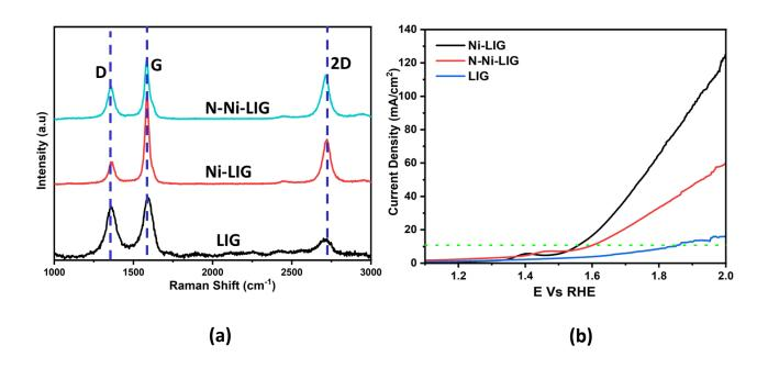
Figure 1: (a) Raman spectra of LIG films and (b) OER polarization curves in 1M KOH with iR correction
