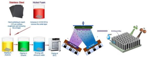
Figure 1 The substrate preparation and deposition of Ni-B-based electrocatalyst coatings with MSPVD
