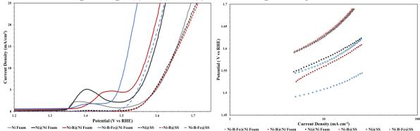
Figure 3 (a)Linear sweep voltammetry (LSV) at the scan rate of 2 mVs<sup>-1</sup> in KOH (1.0 M) solution on MSPVD coatings (b)Tafel plots obtained from LSV curves.
