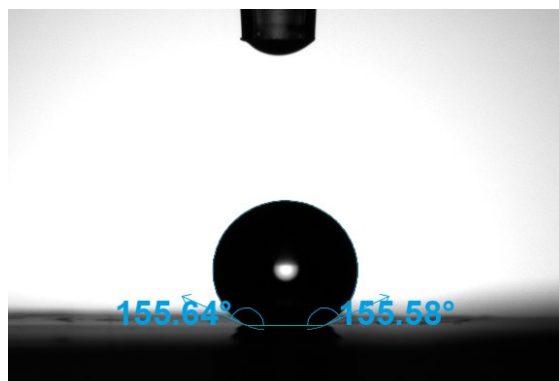
Figure 3. Water contact angle measurement of the antibacterial sample
