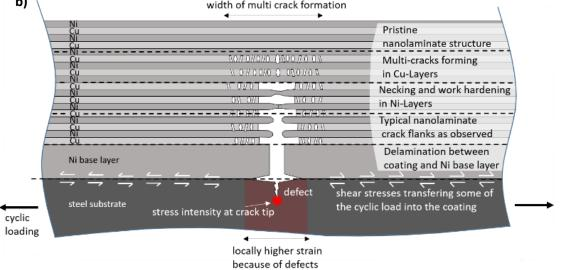
**Figure 1.** a) HAADF TEM image of the crack tip closure in the top part of the TEM-lamella with multicracks forming in the Cu-layers and crack bridging of the Ni-layers; b) schematic crack propagation [5]
