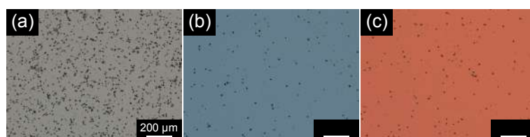
Fig. 4 Images of adherent leukocytes on each sample : (a) NiTi substrate, (b) C 2 H 2 -doped, (c) a-C:H:F with Si-interlayer
