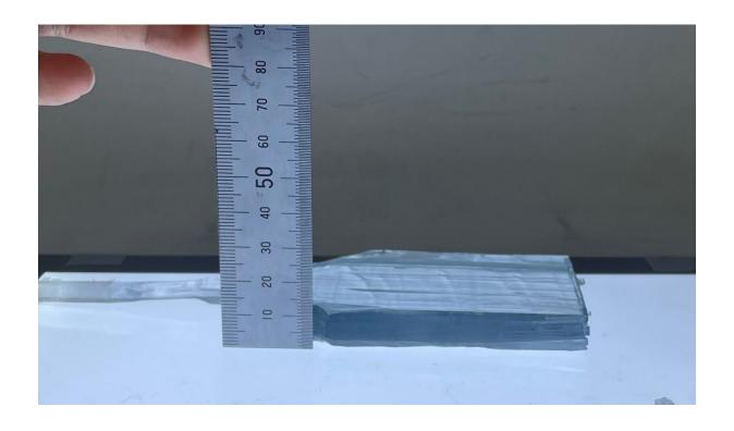
The typical bulk  $Ga_2O_3$  single crystal ribbon grown by EFG method.
