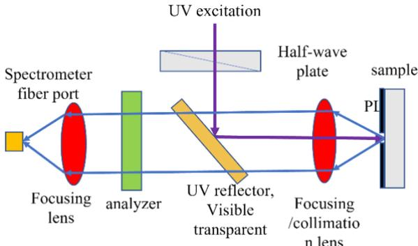
Fig. 1. Schematic of measurement of polarized PL
