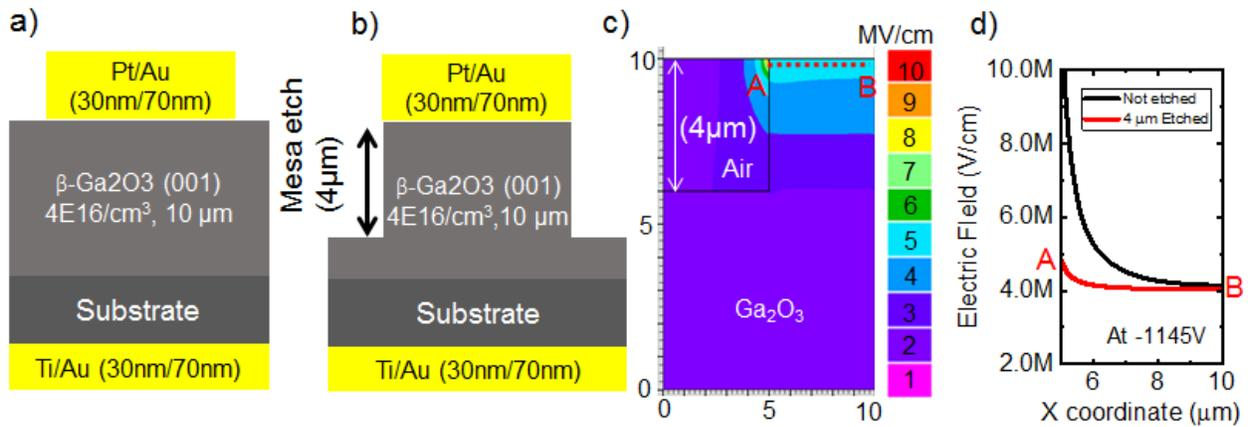
Figure 1: Schematic of (a) unetched and (b) deep-etched devices. (c) 2D electric field simulation of etched device (d) Line plot of electric field along the cut-line (A-B) for etched and unetched devices
