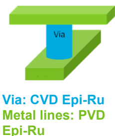
Figure 1. Schematic of epi-Ru interconnects
