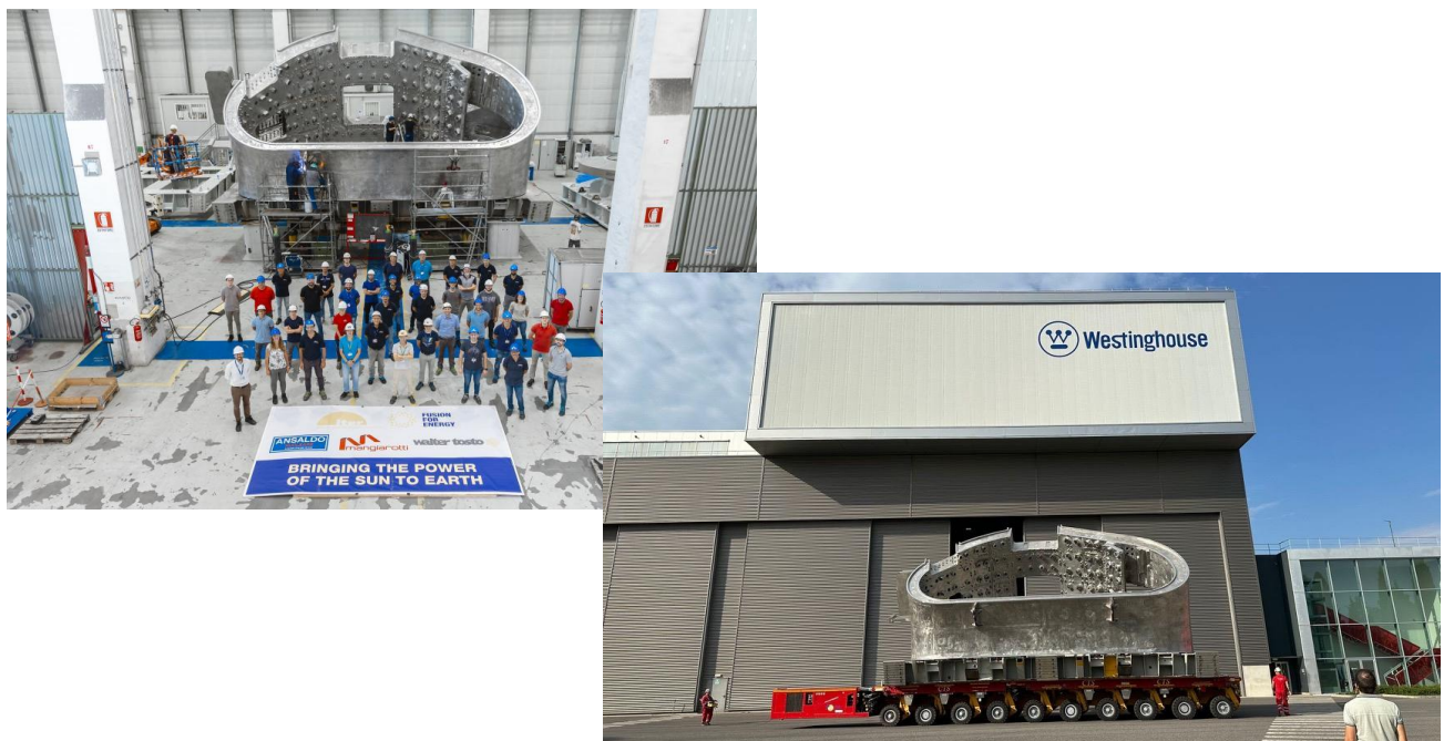
Figure 2: ITER Vacuum Vessel Sector No.5 manufactured by the Ansaldo-Westinghouse-Walter Tosto (AMW) consortium and assembled at the Westinghouse Italy facility
