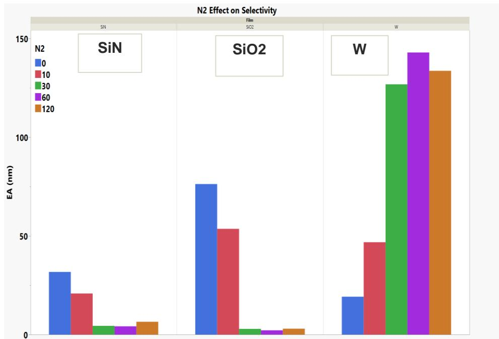
Etch amounts of tungsten, silicon dioxide, and silicon nitride with different nitrogen flow in a BCl<sub>3</sub>/N<sub>2</sub>/Ar plasma.
