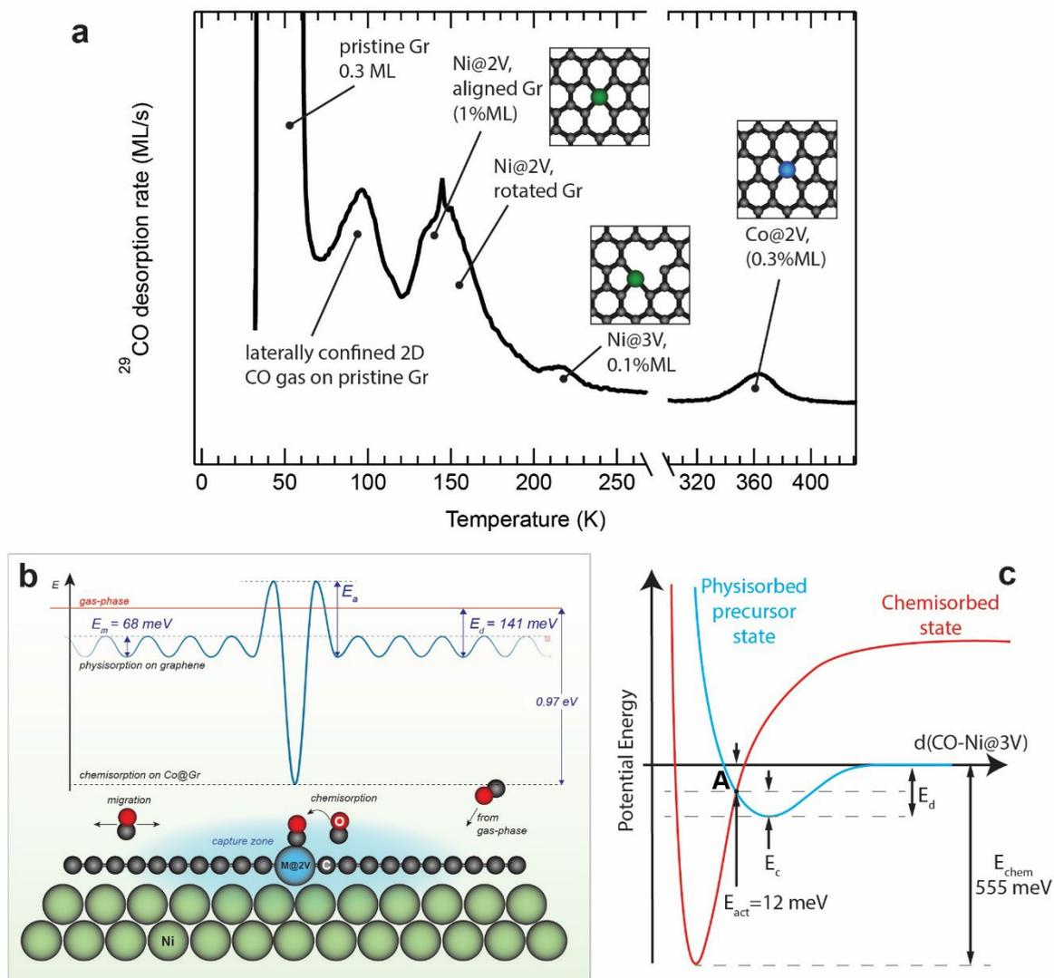
Figure 1: a) CO TPD on a Co and Ni doped Gr/Ni(111) monolayer, and identification of the adsorption sites; b) Energetic landscape of CO adsorption on single metal atoms embedded in Gr di-vacancies (M@2V, M=Ni, Co), after CVD growth on Ni(111). For Co,  $E_a = 174 \text{ meV}$ , while, for Ni,  $E_a \sim 100 \text{ meV}$ ; c) Kinetic model representing CO adsorption on Ni@3V, mediated by the presence of a precursor state.
