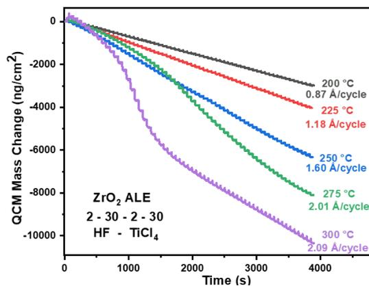
Figure 2. Mass changes during ZrO<sub>2</sub> ALE cycles at 200, 225, 250, 275, and 300 °C with the HF and TiCl<sub>4</sub> with 2–30–2–30 at pressures of 0.6 Torr for HF and 1.2 Torr for TiCl<sub>4</sub>.
