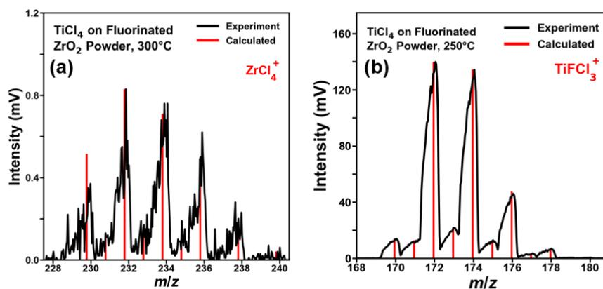
Figure 3. Mass spectrum of the (a) ZrCl<sub>4</sub><sup>+</sup> ion signal and (b) TiFCl<sub>3</sub><sup>+</sup> ion signal during TiCl<sub>4</sub> exposure on fluorinated ZrO<sub>2</sub> powder.
