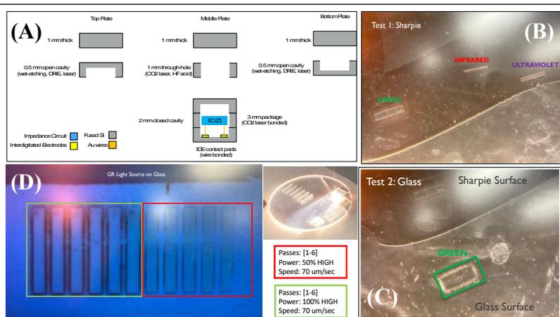
**Fig. 1.** Laser micromachining approach for fused silica material. (A) Hermetic packaging conceptualization using 3 layers of fused silica [5]. Top and bottom layers are micromachined to create a cavity housing the IC and biosensor system. (B-C) Multimodal laser micromachining on fused silica. Green laser source engraved the material surface (D) Green laser micromachining parametrization at 50 and 100% power with a varied number of passes.
