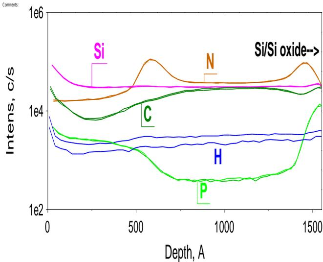
Fig. 1 Two sequential SIMS depth profiles of a 1500Å poly Si on 1000Å Si oxide sample display good repeatability between all elements except for H. The same element in the two sequential profiling is labelled with the same color. All elements are in raw ion counts. The e-beam was applied to overcome the sample charging effects arising from 1000Å Si oxide underneath of the poly Si films
