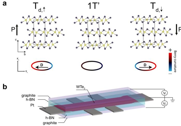
**Fig. 1 Electrical control of stacking order transitions in WTe<sub>2</sub>.** **a**, Side view ( $b$ - $c$  plane) of unit cell showing possible stacking orders in WTe<sub>2</sub> (monoclinic  $1T'$ , polar orthorhombic  $T_{d,\uparrow}$  or  $T_{d,\downarrow}$ ) and schematics of their Berry curvature distributions in momentum space. The yellow spheres refer to W atoms while the black spheres represent Te atoms. **b**, Schematic of dual-gate h-BN capped WTe<sub>2</sub> device.
