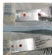
5 μL Blood Drop wetting an Hyper-hydrophilic coating, HemaDrop™ WB. An 8 mm diameter plasma outer ring with 0.75 mm width, and an inner whole blood center with a 6 mm diameter form consistently for each drop tested
