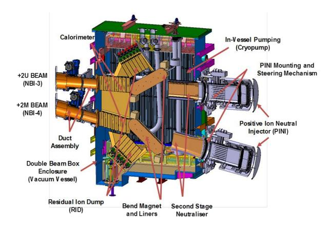
Fig. 1. Sketch of the MAST-U double beamline NBI system design.
