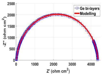
Supplemental data. Nyquist plot of CZTSe Ge bi-layers devices. Impedance Z with Constant phase element (blue) and modelling of EC (red)
