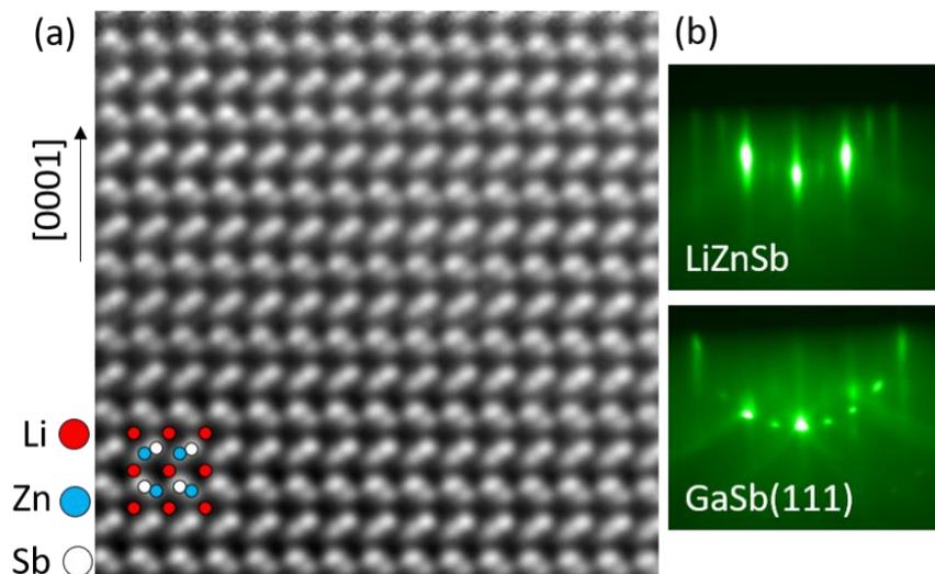
Figure 1 (a) HAADF-STEM image of LiZnSb, showing the polar structure. (b) RHEED patterns for the LiZnSb and GaSb (111) buffer layer.
