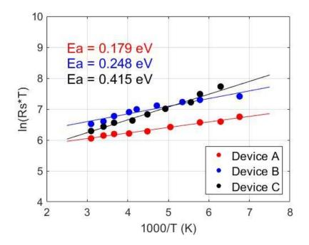
Barrier height extracted from ln(Rs\*T) vs 1000/T plot. The barrier height of device A is improved by 27 % as compared to device B. R-squares for device A (red) is 0.99, 0.93, and 0.98, respectively.
