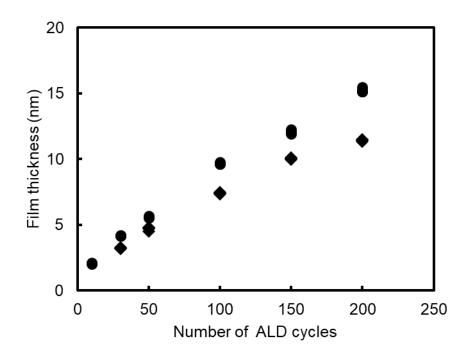
Fig. 1. SnO film thickness as function of number of ALD cycles. The ALD conditions were a  $Sn(EtCp)_2$  pulse time of 10.0 s, a  $H_2O$  pulse time of 3.0 s, and a growth temperature of 200 °C.  $H_2$  plasma pulse times were 5 s ( $\blacksquare$ ) and 1 s ( $\spadesuit$ ), respectively.
