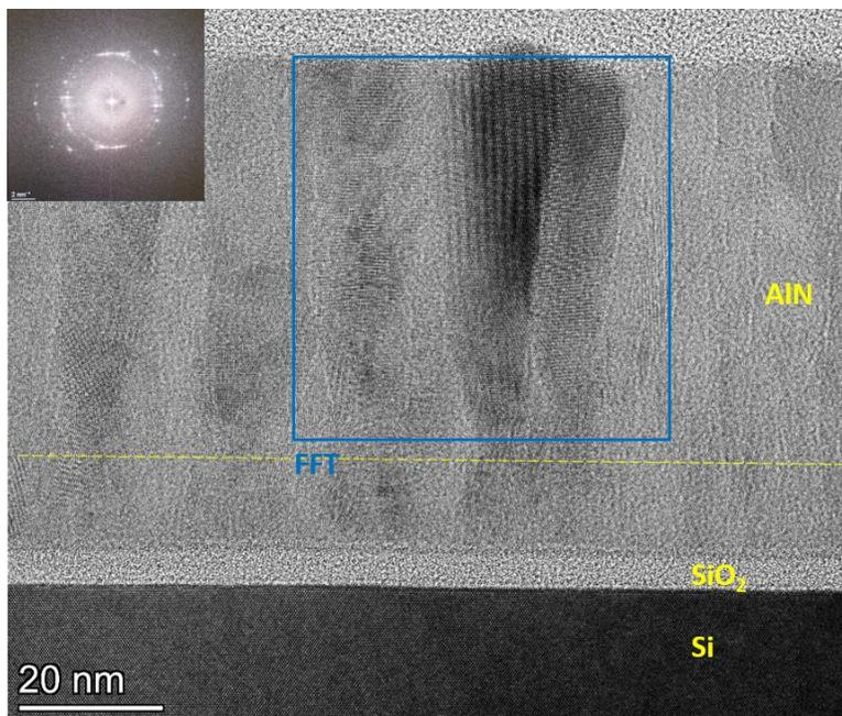
**FIG.5. HR TEM micrograph and FFT analysis** (inset) of AlN film grown on SiO<sub>2</sub>/Si substrate. AlN thickness is ~ 66 nm. The AlN grows poorly textured up to the layer thickness of ~ 20 nm. Highly textured columnar growth of AlN is observed when the layer thickness becomes greater than 20-25 nm.
