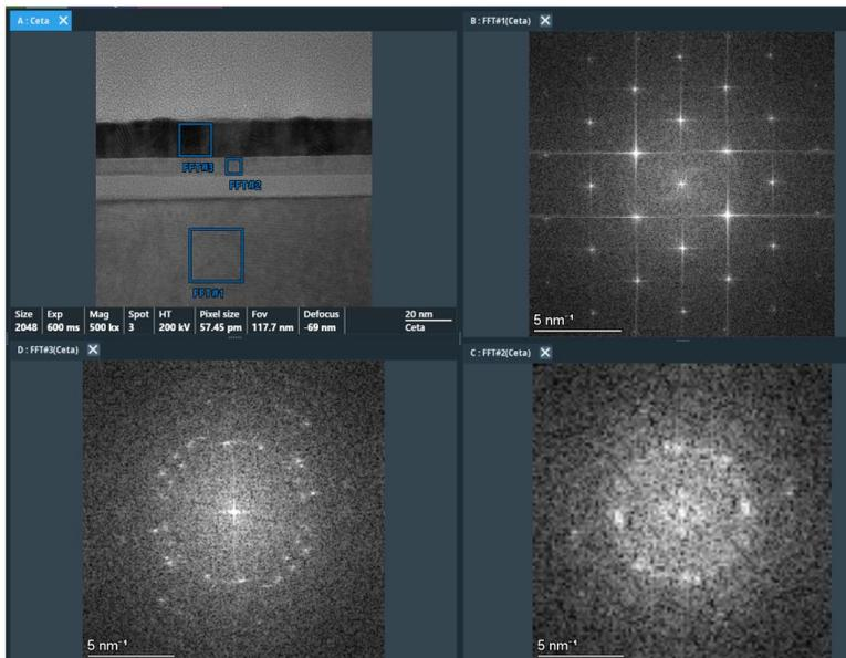
**FIG.3. HR TEM micrograph and FFT analysis** of TiN/AlN film grown on SiO<sub>2</sub>/Si substrate. AlN layer thickness is about 8 nm. FFT1, FFT2, FFT3 are taken from the areas marked on TEM image: FFT1 – Si substrate; FFT2 – AlN layer; FFT3 – TiN layer. AlN grown on an amorphous substrate is poorly textured. TiN is almost not structurally related to AlN IL, the extent of texturing is low.
