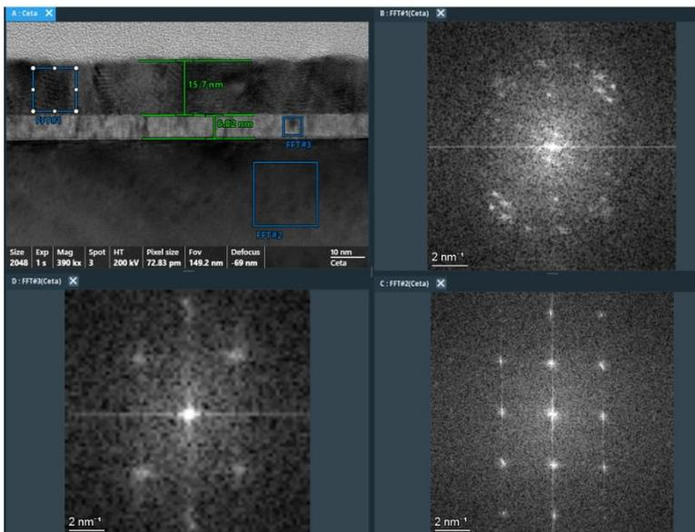
**FIG.4. HR TEM micrograph and FFT analysis** of TiN/AlN film grown on a sapphire substrate. AlN layer thickness is about 7nm. FFT1, FFT2, FFT3 are taken from the areas marked on the TEM image: FFT1 – TiN layer; FFT2 – sapphire substrate; FFT3 – AlN layer. AlN is perfectly aligned with the sapphire substrate, is highly textured and almost single crystalline. TiN is structurally related to AlN IL and sapphire, textured as well. It preserves mosaicity of ~15 nm grains.
