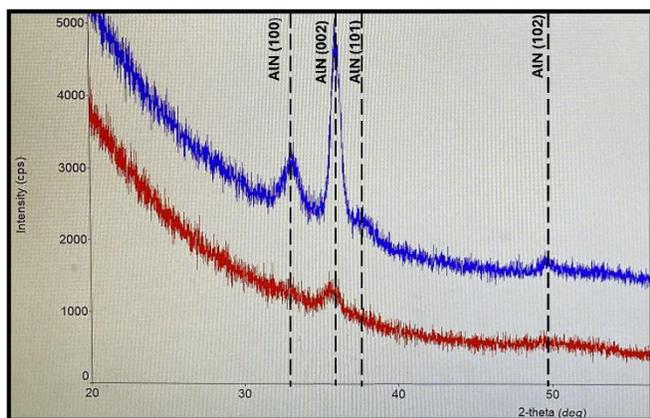
**FIG. 1. XRD spectra** measured using grazing incidence angle XRD scan mode ( $\omega = 0.5^\circ$ ) of AlN layer deposited by PEALD (N<sub>2</sub>/Ar plasma, power 300 W, at 300 °C, TMA precursor). Red line – 12 nm AlN thickness; blue line – 66 nm AlN thickness. The peaks of hexagonal AlN are marked. Increasing the AlN thickness leads to better texturing of the film, which is indicated by rising and narrowing of the XRD peaks.
