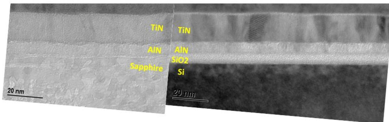
**FIG.2. BF TEM micrographs** of the TiN/AlN films grown on SiO<sub>2</sub>/Si substrate (right) and on sapphire substrate (left) with N<sub>2</sub> plasma. Sapphire substrate initiated epitaxial-like growth. In the case of SiO<sub>2</sub>/Si substrate AlN layer is much less uniform, growth of TiN is less related to AlN
