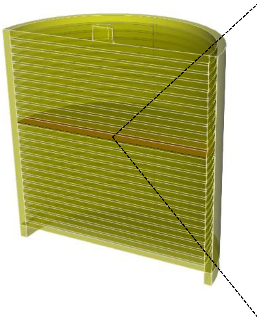
Fig. 1. ALD reactor model scheme
