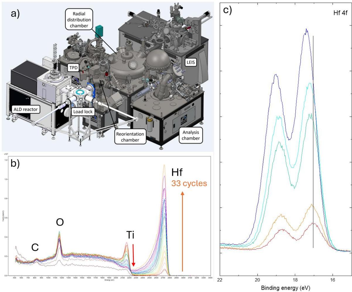
Figure 1. a) HelsinkiALD cluster tool, b) LEIS spectra up to 33 cycles of HfO<sub>2</sub> deposition on TiN, c) Hf 4f XPS spectra of 5, 10, 30, 40, 50 cycles of HfO<sub>2</sub> deposited on TiN. The line on the spectra indicates the binding energy shift which varies with the number of deposition cycles.
