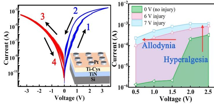
Fig. 1. (a) I–V curves of the Pt/Ti-Cys/TiN device for 100-cycle DC ramped voltage tests. The schematic of this hybrid device is shown in the inset. (b) The maximum output currents in log scale at 2 ms voltage pulses with different amplitudes after different injury pulses.
