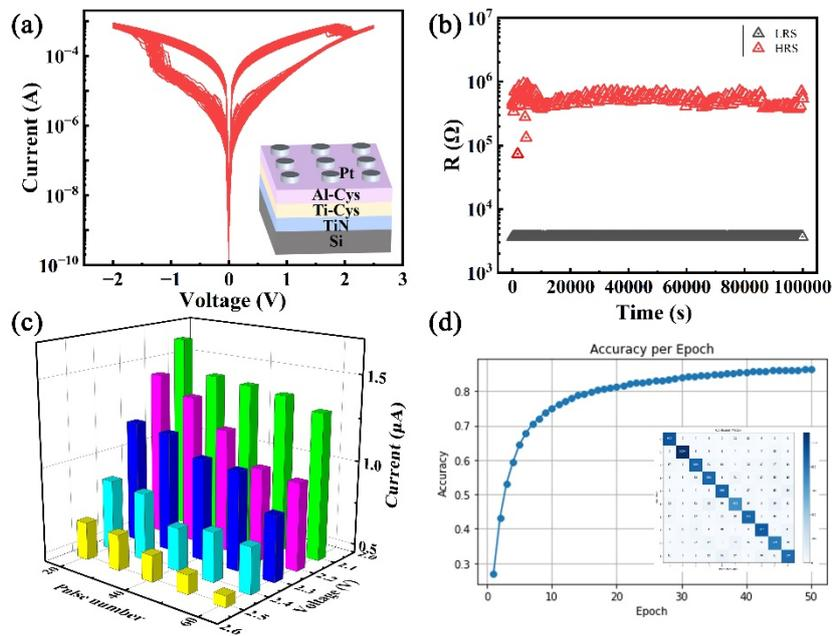
Fig. 2. (a) I–V curves for 100 tests with the schematic of the bilayer Pt/Al-Cys/Ti-Cys/TiN memristor device. (b) Retention of the bilayer memristor for  $10^5$  s. (c) Response of a memristor device to different pulse programs. (d) Training epoch-dependent recognition accuracy and the confusion matrix.
