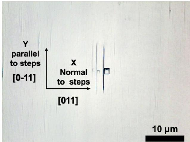
Figure 1: Polished (100) diamond surface post-treatment with H plasma, showing crystallographic etching of defects induced during traditional polishing processes.
