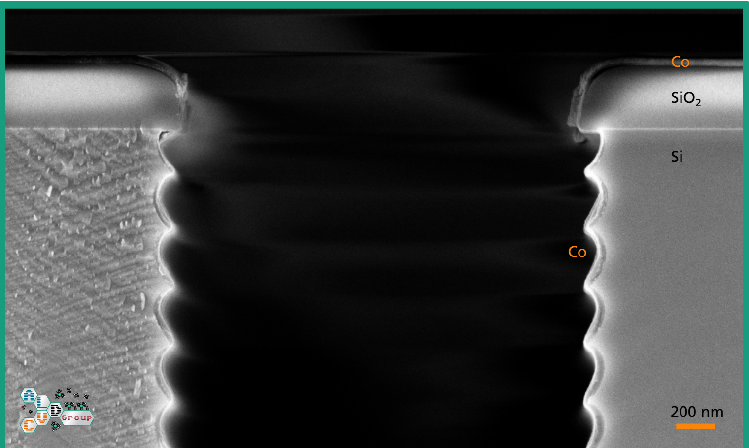
Figure 2: Scanning Electron Microscopy image of trench testing structure with cobalt coating.
