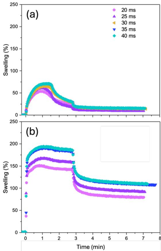
**Figure 1.** Swelling of PMMA (a) and PLA (b) films during the SIS process. Different curves were obtained changing the length of the TMA pulse.
